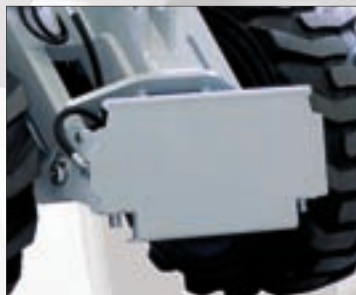
Automatic attachment coupling plate
